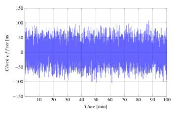
(a) Readings of the measured clock offset between TSN Evaluation Kit and Intel NUC mini PC over time.
