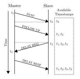
Fig. 1. Message exchange and corresponding timestamps in PTP (IEEE 1588).
