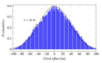
(b) Histogram of the probability density functions obtained for the readings of the clock offset.
