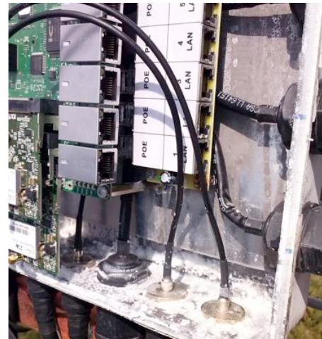
Fig. 2. Transmitter damaged by humidity (Mbachile base station)
