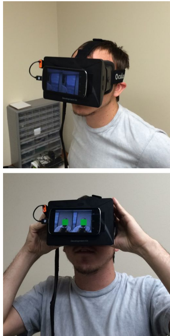
Fig. 1. Student with prototype based on the Oculus Rift headset. The hardware in this demo was suitable for both virtual and augmented reality development (thanks to the on-board phone's camera being used to supply the main video feed to the headset), but costs over $600, took several hours to assemble, and was generally unwieldy in use.
