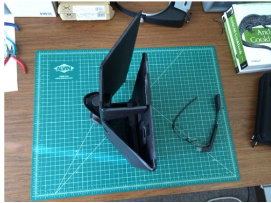
(d) A side view of a completed device, this one prepared for a small screened device. In this instance, it was a large smartphone, but larger devices can be accommodated by adjusting the distance between the device and the eyepieces.
