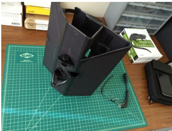
(e) An angled view of the device, showing more clearly how it is simply a folded portion of a foam board intended to hold an electronic screen at a fixed distance from the eyepieces.
