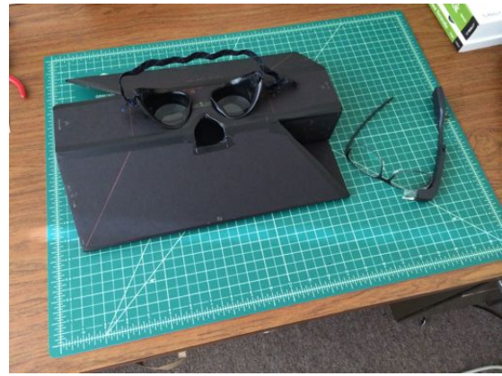
Fig. 3. The DIY goggles compared against Google's Glass. Both require a smartphone, but the DIY goggles we constructed on the left were constructed in under an hour using less than $12 of simple materials. Google glass is a more capable and wearable device, but would cost a developer over $1,500 to purchase (placing such technology well outside the reach of most students, particularly in developing countries). The DIY version, while unwieldy, was found to be more convenient for experimentation and less unwieldy than the earlier development prototype, which had been built around the Oculus Rift (and shown in Figure 1).
