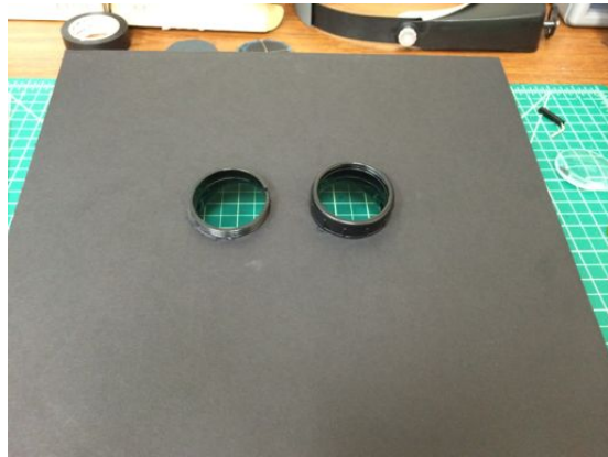
(b) Attaching goggles to foam board using the threaded lens frames.
