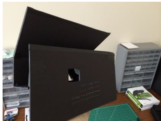
(f) A view of the side opposite the eyepieces. In this instance, the backing was cut to accommodate the rear camera of the phone being used.
