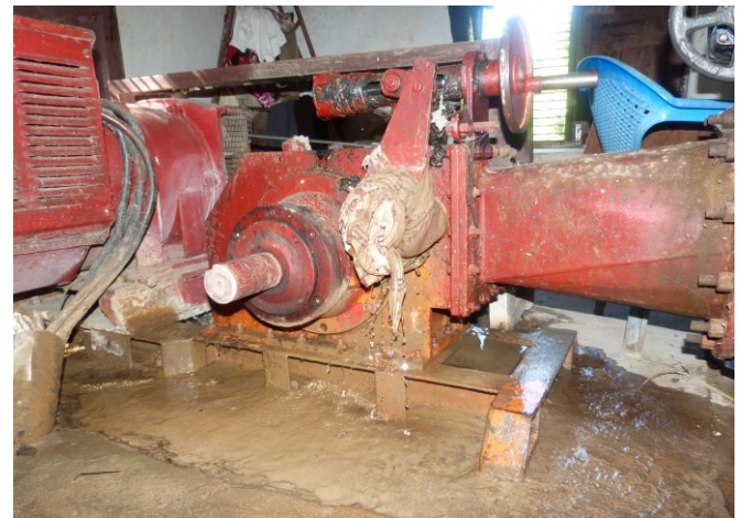
Fig. 6 Leakage from turbine casing
