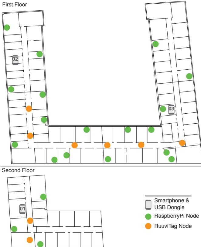
Fig. 4: Proof-of-concept setup for the smart office experiments.
