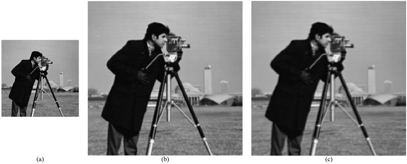
Fig. 8. The final results (a) Input image (b) Result of the bilinear interpolation (c) Result of the bicubic interpolation
