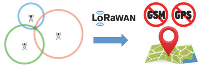
Fig. 1. LoRaWAN geolocation based on time of flight analysis of the packages sent from a low power IoT device. No GPS or GSM units were used.
