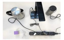
Fig. 7. Devices used in the demonstration. Bottom left: homee gateway, top (left to right): kettle and desk lamp connected to 2 Fibaro Wall Plug, Amazon Echo
