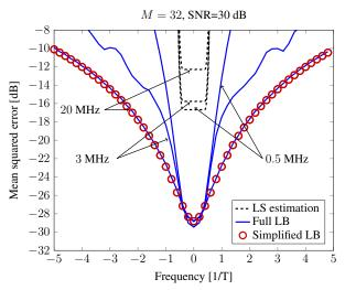
Fig. 5. As opposed to SISO systems, for SIMO systems, the rays can be separated much more easily in the delay-angle domain, implying that (As2) becomes valid much faster. The maximal extrapolation gain is already attained for 1/T = 20 MHz while achieving an additional SNR gain.
