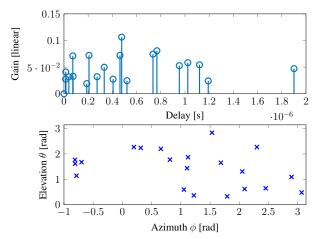
Fig. 2. Generated set of parameters  $(\alpha_l, \tau_l, \phi_l, \theta_l)$  for l = 1, ..., L - 1 with L = 21 and following 3GPP 3D-UMa NLOS model. The sum of gains is normalized to one.
