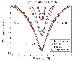
Fig. 3. The SAGE algorithm can reach the performance of the full LB (Theor. 1). The simplified LB (Corol. 1) gets closer to the full LB as the number of antenna increases meaning that (As2) is better validated: the rays are more separated in angle. We also notice a large SNR gain with respect to conventional LS.
