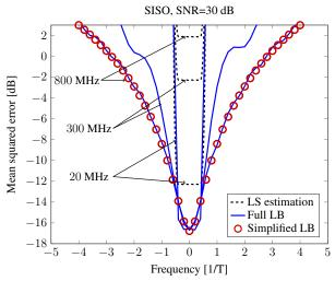
Fig. 4. As the bandwidth increases, extrapolation becomes possible in SISO and the full LB converges to the simplified LB meaning that (As2') holds. A bandwidth of 1/T = 800 MHz is necessary for (As2') to be completely valid.
