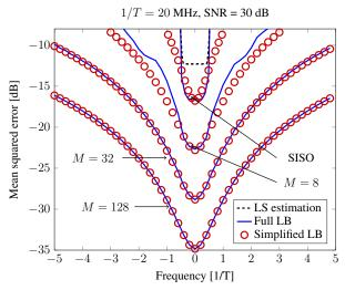
Fig. 6. As the number of antenna elements increases, the rays can be more easily separated in the angle domain and the full LB converges to the simplified LB.
