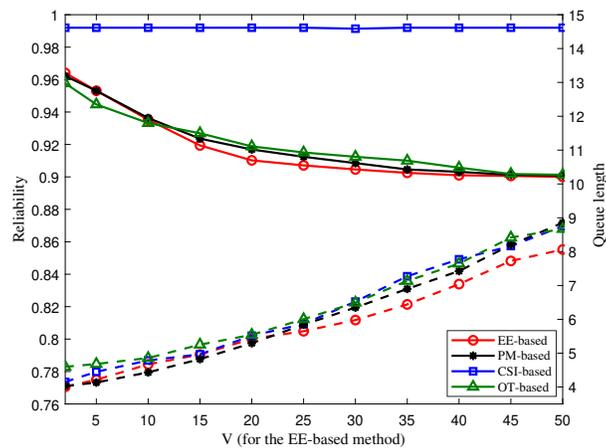
Fig. 3. Average reliability of type-1 messages (solid lines) and average queue lengths of type-2 messages (dashed lines).
