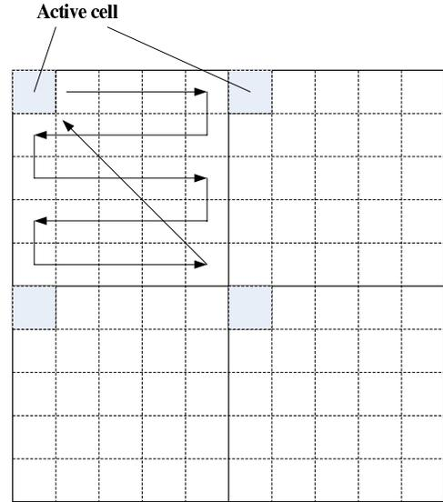
Fig. 1. A four-cluster example with 25 cells per cluster. The cells in each cluster take turns to be active along the arrowed line over time.
