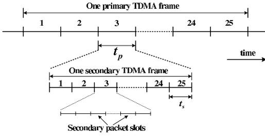
Fig. 4. Structure of the secondary TDMA frame and its relationship with the primary TDMA frame, where  $t_s$  is the time-slot duration for the secondary TDMA scheme.
