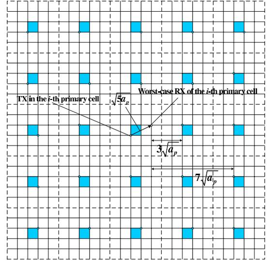
Fig. 8. Interference from the concurrent primary transmissions to the worst-case primary RX of the transmission from the  $i$ -th primary cell.
