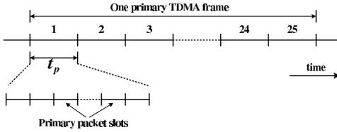
Fig. 3. Structure of the primary TDMA frame, where  $t_p$  is the time-slot duration of the primary TDMA scheme.
