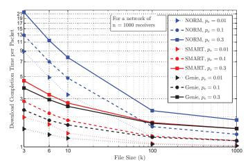
Fig. 7. Simulation results depicting the performance of SMART, the theoretical bound obtained from a genie based protocol, and a wireless representation of NORM.
