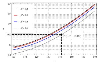
Fig. 6. The number of nodes n that can be accommodated for a given transmission time t. The figure was computed according to (12) with k=100 packets and  $p_e=0.1$ . An example of how the time  $t^*\left(\beta^*,n\right)$  can be obtained from these curves is illustrated by the dashed lines for the case of  $\beta^*=.9$  and n=1000.
