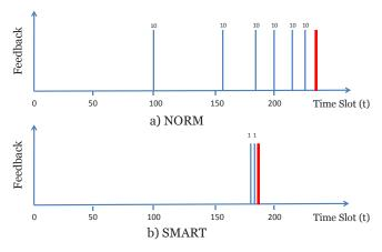
Fig. 1. Feedback times for NORM vs. SMART for n=10000, k=100, and  $p_e=0.3$ . The number above each blue bar indicates the number of slots devoted to NACKs at that cycle and red bars denote the end of transmissions.
