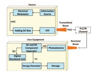
Fig. 1. SLIPT transceiver design
