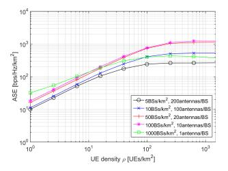
Fig. 2. The ASE performance of different antenna deployment when  $\gamma_0=0\,\rm dB$  vs. UE density  $\rho$  with 1000 antennas/km^2
