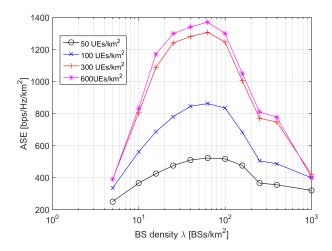
Fig. 4. The ASE performance without pilot contamination of different UE density when  $\gamma_0 = 0 \text{ dB vs.}$  BS density  $\lambda$  with 1000 antennas/km<sup>2</sup>
