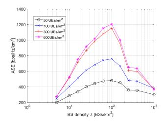
Fig. 3. The ASE performance of different UE density when  $\gamma_0 = 0 \, dB$  vs. BS density  $\lambda$  with 1000 antennas/km<sup>2</sup>
