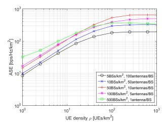
Fig. 1. The ASE performance of different antenna deployment when  $\gamma_0=0\,{\rm dB}$  vs. UE density  $\rho$  with 500 antennas/km^2
