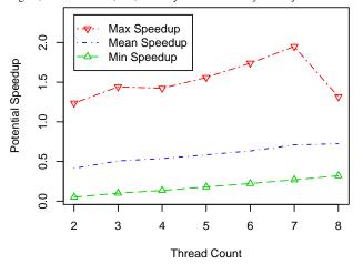
Fig. 3. Potential scalability for XML input encoding an array of 50,000 Mesh Interface Objects. The number of threads available is the independent variable here. A slight speedup is possible by adding more threads for this class of input.
