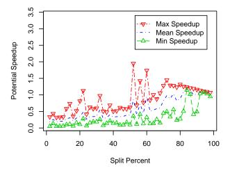
Fig. 4. Similar to figure 3, this graph presents the result on speedup of varying the split percent parameter when processing an encoded array of 50,000 Mesh Interface Objects. Maximal and minimal speedups for each selection of split percent are shown. The range of values comes from varying the number of threads.
