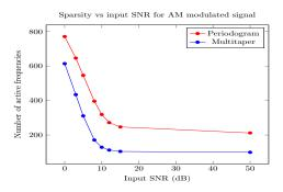
Fig. 6: Effect of MT method on signal sparsity verses input SNR for an AM modulated signal.
