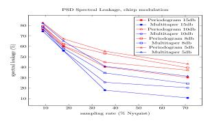
Fig. 2: PSD spectral leakage performance of the *MT-RD* and periodogram for the chirp test signal and various input SNR.
