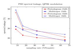
Fig. 7: The effect of MT method on PSD spectral leakage of QPSK test signal for various input SNR.
