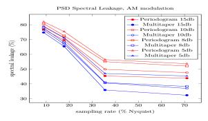
Fig. 3: PSD spectral leakage performance of the *MT-RD* and periodogram for the AM test signal and various input SNR.
