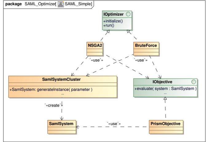
Fig. 4. Simplified software architecture of the SAML optimizer
