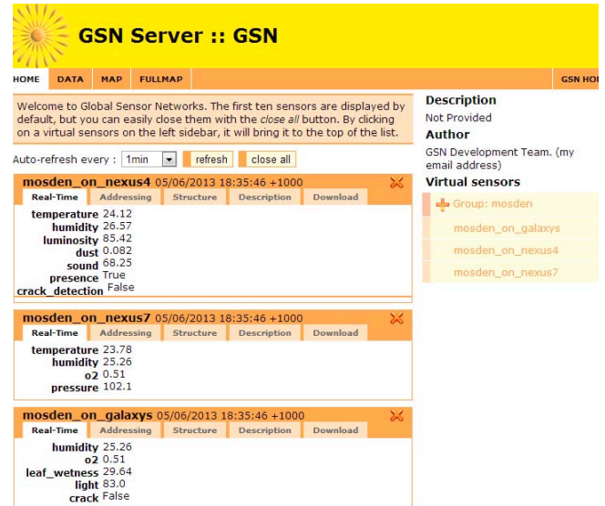
Fig. 6: Screenshot of a cloud GSN instance showing three different MOSDEN instances registration
