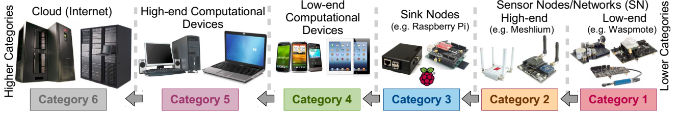
Fig. 1: Categorization of IoT devices based on their computational capabilities. The devices belong to each category has different capabilities depending in term of processing, memory, and communication. They are also different in price where devices becomes more expensive when move to left. The computational capabilities are also get increased when move to left.
