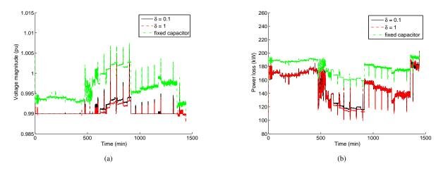
Fig. 6. Real-time traces of (a) voltage magnitude and (b) power loss for different  $\delta$ , and a benchmark case with only a fixed capacitor and no control.
