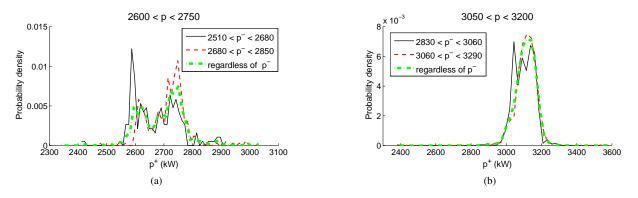
Fig. 3. Examples of probability density of  $p^+$  conditioned on p and  $p^-$ . Subfigures (a) and (b) are for different p, and the legends label different  $p^-$ . To collect sufficiently many samples to plot the probability density, p and  $p^-$  are taken as some ranges as opposed to numbers.
