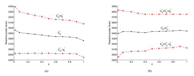
Fig. 5. Sizes of control devices as functions of  $\delta$ . The range of aggregate reactive power injection of the fixed capacitor and the D-STATCOM is plotted for (a)  $c_s = 0$  and (b)  $c_s = C_s^*$ , respectively.
