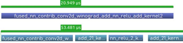
Fig. 5. Fusion saves time by reducing kernel switching overhead. Top: *winograd\_conv2d\_kernel2* is fused with add and ReLU kernel. Bottom: *winograd\_conv2d\_kernel2* is issued separately from add and ReLU kernels, resulting in significant increase in execution time.
