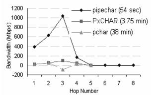
**Figure 5**: NCS, PxCHARand pchar results for a broken network path
