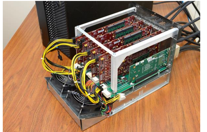
Fig. 7. FPGA prototype of the graph processor.
