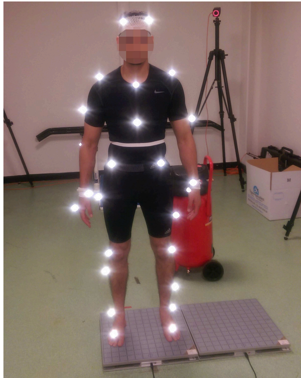
Figure 4.13: The VICON/AMTI-OR6 setup during the experimental phase shows the static body (red object not currently on the force plates used to assist in producing various number of postures while being fixed in one location on top of the force plate surface) and placement of the 35 passive markers following the Plug-in-Gait (PiG) template to define the body segments.
