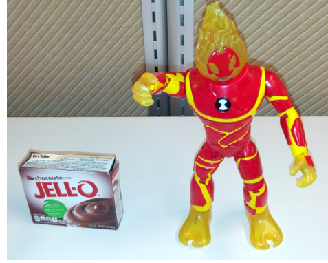
Fig. 4: Shows the two test objects used in the grasping experiment. The robot could only grasp the toy at specific heights from the smaller edges, whereas the box was graspable at all heights from shorter edges.
