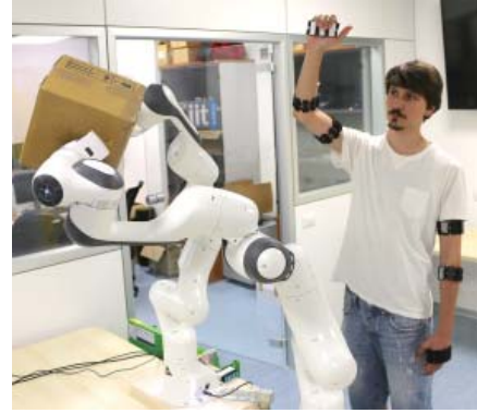
Fig. 1. An example frame of single-arm synergistic manipulation operated with the proposed approach.
