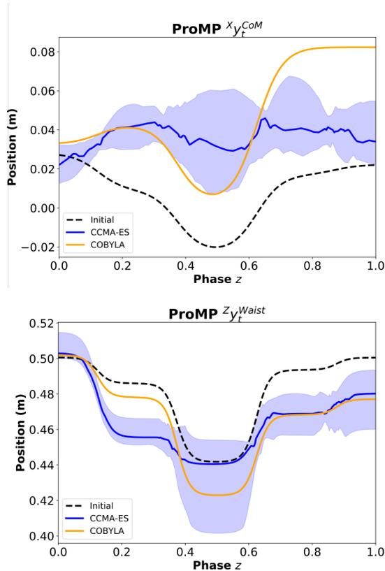
Fig. 8: Reference trajectories: initial (from human demonstrations) and after optimization. Both CCMA-ES and COBYLA were bootstrapped from a ProMP that combined every demonstration, *all*. The 30 reference trajectories for CCMA-ES are represented with their median and IQR.
