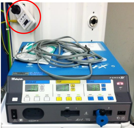
Fig. 1: Electrosurgical device and current sensor (encircled)
