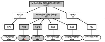
(b) The second chunk after the insertion of 'c' splits into two due to 10 chunk boundary rule. The new chunk's changes are localized as parent 11 node is only determined by h(C) and h(D).
