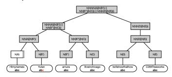
(b) The second chunk in Figure 2a after the insertion of 'c' splits into two due to chunk boundary rule. The new chunk on content "amura**abc**" shifts the hash values and changes the previous Merkle tree almost entirely.
