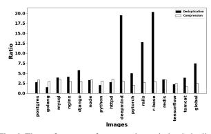
Fig. 6: The performance of compression ratio by deduplication and gzip compression algorithm on individual images.
