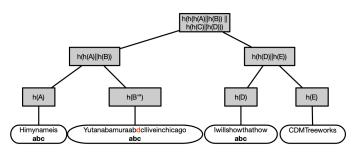
(c) The Merkle tree also changes entirely if the boundary rule is modified. Figure shows the Merkle tree when 'd' is inserted within the boundary rule of second chunk of Figure 2a.
