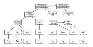
Fig. 5: Versioning due to layering for  $f_1$  and versioning due to branching for  $f_2$ . Layering leads to new hash versions in internal nodes. Branching leads to new hashing nodes.
