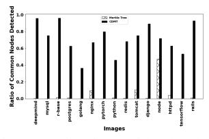
Fig. 8: The comparison of the CDMT index and Merkle Trees generated for the same versions, averaged over all images. CDMT indexes for two versions have higher ratio of common nodes detected because nodes are not cut due to the chunk shift problem as in Merkle Trees.
