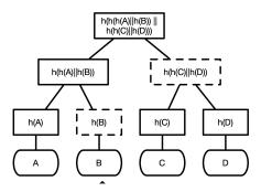
Fig. 1: A binary Merkle tree. The authentication path for leaf at index 0 is shown in dashed nodes
