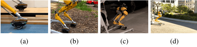
Fig. 9: Cassie riding the Hovershoes on (a) different heights, (b) rough terrain, (c) up a 7^\circ incline, and (d) down a 13^\circ incline.
