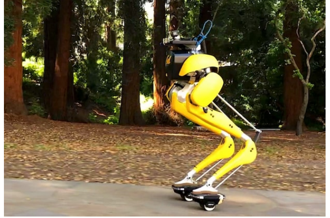
Fig. 1: Snapshot of an experiment of the bipedal robot Cassie autonomously riding on Hovershoes. Experimental videos are at https://youtu.be/b2fKBb.0iTo .
