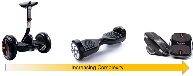
Fig. 2: Segway, Hoverboard, and Hovershoes are shown from left to right. The complexity in terms of user control increases along the arrow head direction.
