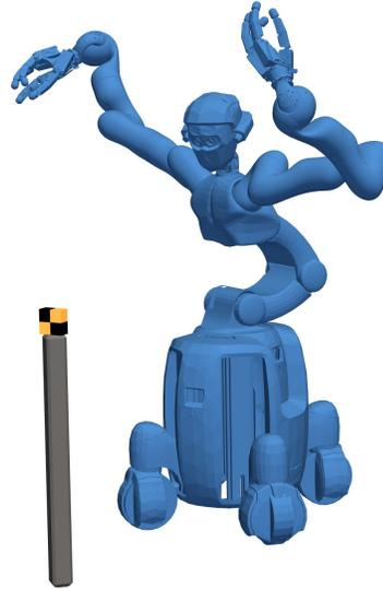
Fig. 1. DLR’s Agile Justin [2] collecting measurements using its head-mounted RGB camera for the calibration of its elastic forward kinematics as well as the camera’s intrinsic and extrinsic parameters. Only simple markers on both hands as well as the depicted marker mounted on a pole are used. As described in Section V, we select filtered random configurations to identify the robot in its whole work space.
