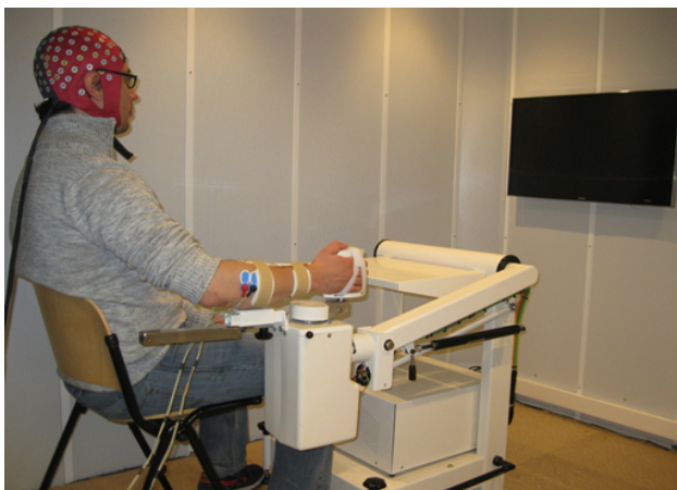
Fig. 1. Experimental setup. The right forearm of the subject is strapped into an armrest and the right hand is strapped to the handle, requiring no hand force to hold the handle. Both angle of and torque at the axis of the motor are recorded.
