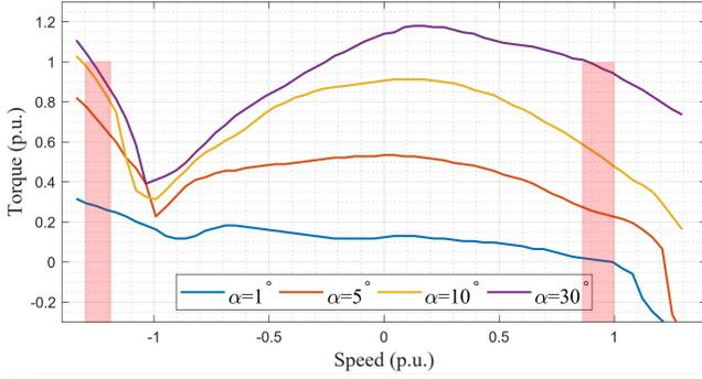
Fig. 2. Torque speed characteristics of a typical reversible pump turbine at different guide vane openings ( $\alpha$ ). The speed is positive in generating mode and negative in pumping mode. The shaded region shows the rated operating region. Courtesy: Water Power Laboratory, NTNU, Trondheim.
