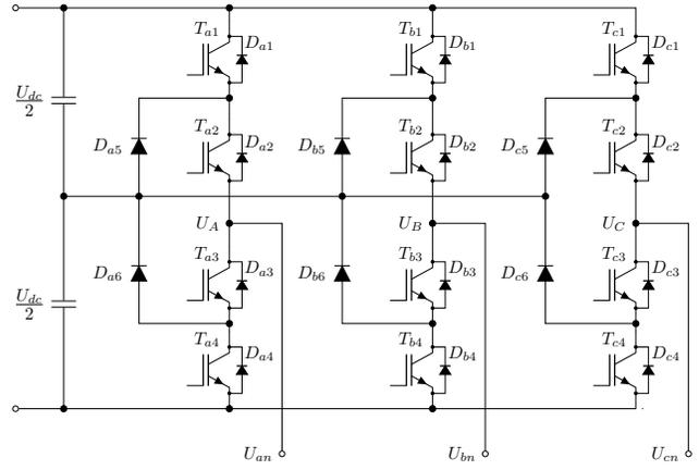
Fig. 3. Schematic of a 3-level 3-phase Neutral Point Clamped (NPC) Converter configuration.
