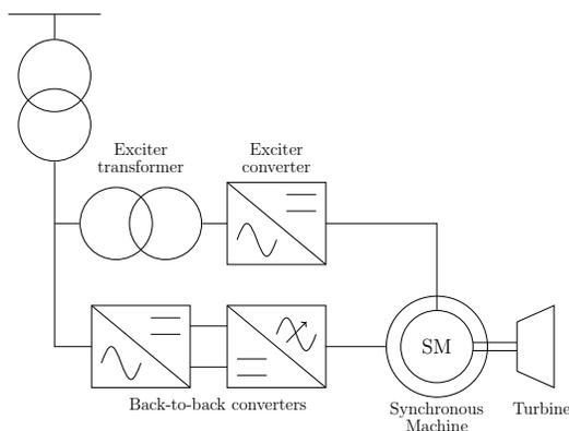
Fig. 1. Schematic of Converter Fed Synchronous Machine Technology.
