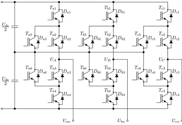
Fig. 4. Schematic of a 3-level 3-phase Active Neutral Point Clamped (ANPC) Converter configuration.
