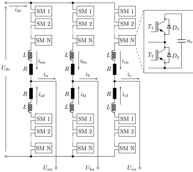
Fig. 5. Schematic diagram of a Modular Multilevel Converter with half-bridge sub-module configuration. A typical dc link voltage of 22 kV and ac output voltage is 13–15 kV (rms). In this figure, "SM" stands for Sub-module.
