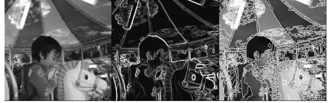
Fig. 1. A gray tone image, its gradient and the watershed segmentation associated to the minima of the gradient.
