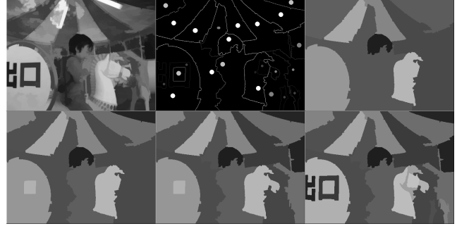
Fig. 4. A number of prioritized markers have been chosen: they appear as disks whose shade of grey is brighter for higher priorities. The associated hierarchy is illustrated through the saliency of the contours in the second image and through 4 levels of the associated hierarchy.
