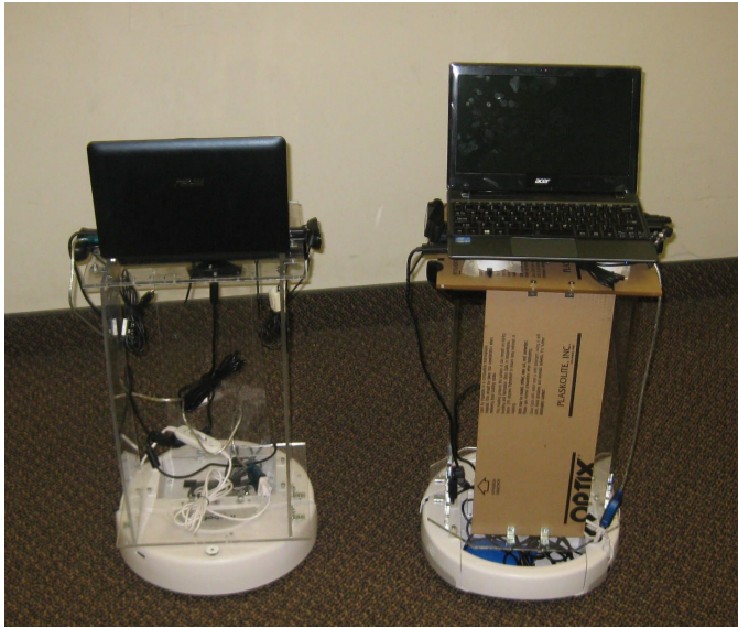
Fig. 2. The first two corobot prototypes, which differ only slightly in their construction. The first prototype (on the left) is facing toward the camera, while the other is facing away.
