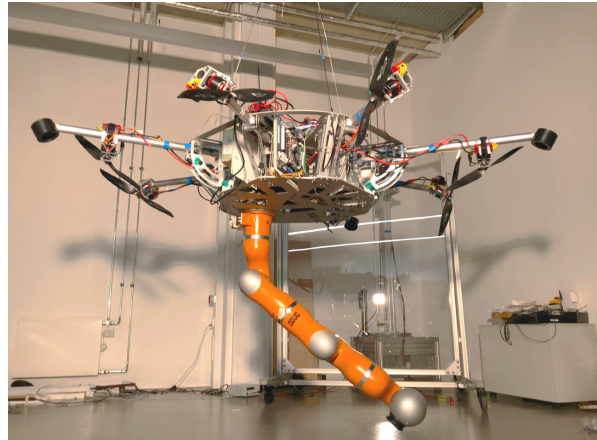
Fig. 1: DLR Suspended Aerial Manipulator [13], whose model was used to validate the proposed approach.
