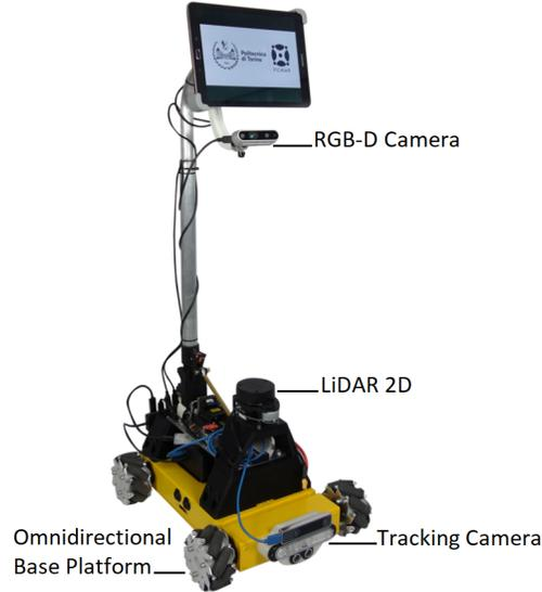
Figure 2: The omnidirectional platform we set up for experimentation and validation of our novel methodology.
