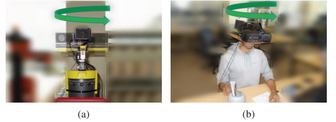
Fig. 5: (a) The movement of the Kinect camera, determined by the head movements of operator. (b) The natural head movements of the operator, tracked by the headsets built-in IMU.
