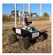
Fig. 5: Summit XL Robotic platform, including the equipment used in the challenge.
