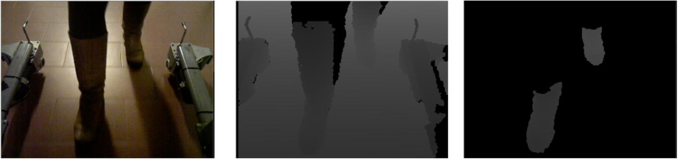
Fig. 2. Frames depicting different aspects of the markerless method proposed in this work. *Left*: Color frame (from the RGB sensor) shown to the user for visual feedback; *Center*: Depth frame after background subtraction; *Right*: Left and right feet after segmentation;
