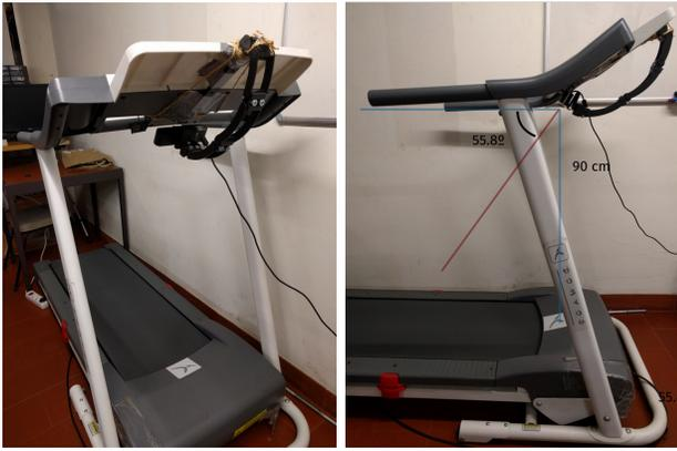
Fig. 3. An Orbbec Astra camera was installed under the treadmill control panel, at a height of 90 cm and aligned with the start of the walking mat/zone, at an angle of  $55.8^\circ$  with the walking surface. This setup found empirically to allow both feet to be within the camera's *FoV* during the entirety of the walking cycle.
