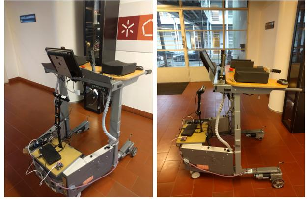
Fig. 4. The *ASBGo Smart Walker* on a university setting (straight corridor used for validation trials). Camera installation is the same as Figure 3.
