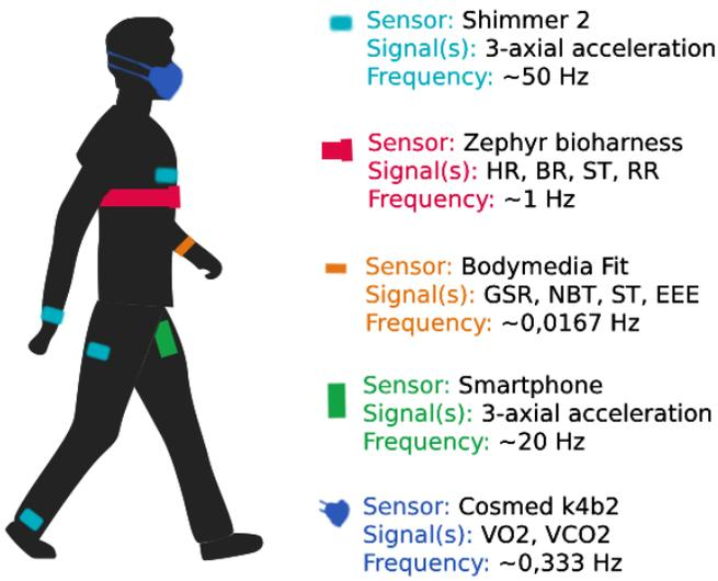
Fig. 2: Representation of on-body location of the sensors, measured signals, and the corresponding acquisition frequency.
