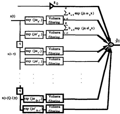
Fig.6.-The K-filter to model NLSs with memory.
