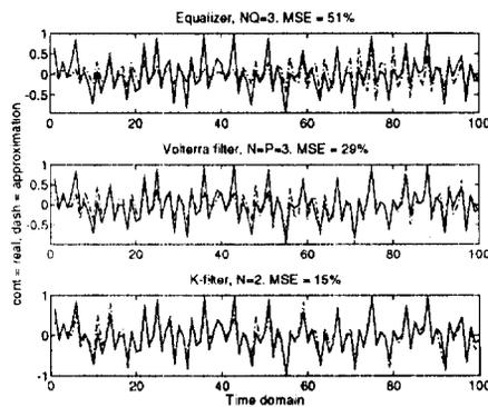
Fig.7. Results of the simulations. The first one corresponds to an equaliser, the second one to a Volterra filter with memory and the third one to the K-filter.
