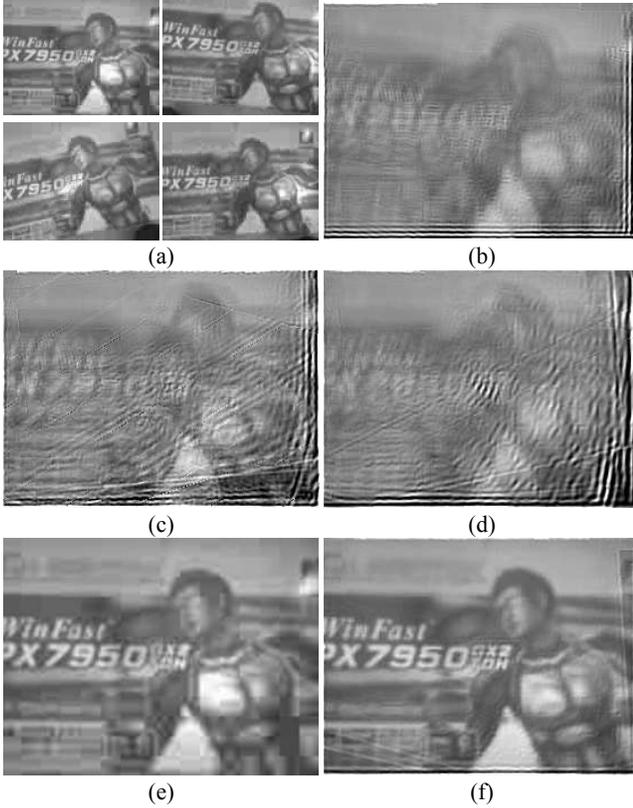
**Fig. 3.** (a) various LR frames (4 out of 8 used) of a video with spatially varying illumination captured using a mobile phone camera; SR reconstruction results using different registration algorithms (b) intensity minimization (c) RANSAC (sift point detector) (d) RANSAC (Harris point detector) (e) single frame bicubic (f) phase-based method; compression artifacts is absent in (f) and the center text is more clear
