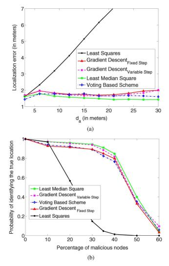
Fig. 6. Performance of the secure localization schemes under coordinated attacks by 30% of the nodes. (a) Average localization error and (b) probability of correctly identifying the true position for  $d_a = 22$  m.
