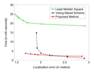
Fig. 3. Comparison of run-time for different localization schemes for a fixed localization error.
