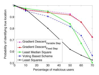
Fig. 5. Probability of converging to the correct estimate for different localization schemes under noncoordinated attacks for  $\sigma_{\rm attack} = 4$  m.
