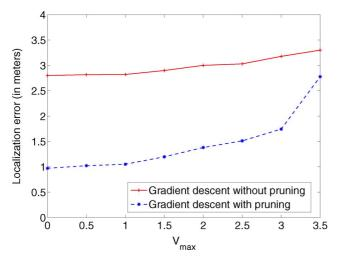
Fig. 13. Effect of velocity on the error in estimating the map of relative locations.
