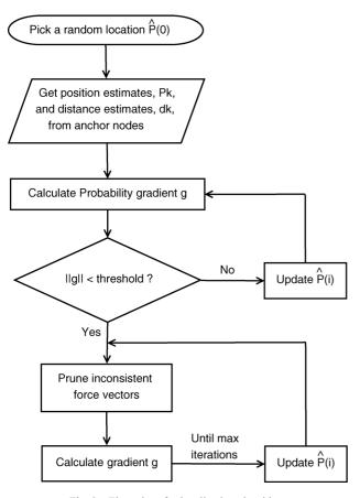
Fig. 2. Flow chart for localization algorithm.
