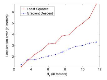
Fig. 10. Localization accuracy for coordinated attacks by 30% of the nodes using TDoA measurements.
