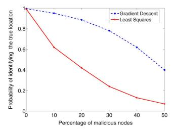
Fig. 11. Probability of converging to the correct estimate under coordinated attacks for TDoA,  $d_a = 22$  m.
