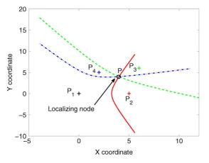
Fig. 9. Intersection of three hyperbolas gives the location of a node when TDoA is used.
