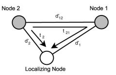
Fig. 8. Diagram representing the basic TDoA protocol.
