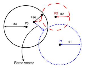
Fig. 1. Force vector representation of terms contributing to the gradient.
