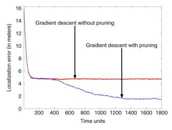
Fig. 12. Localization error, E(t), as a function of time for estimating the relative locations in MSNs when 50% nodes are malicious.
