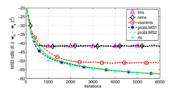
**Fig. 1**. Performance in terms of MSD of probabilistic LMS with both optimal (probLMS1) and suboptimal (probLMS2) compared to LMS, NLMS, VS-LMS, and RLS.
