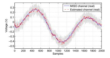
**Fig. 2**. Real part of one coefficient of the measured and estimated channel in experiment two. The shaded area represents two standard deviations from the prediction (the mean of the posterior distribution).
