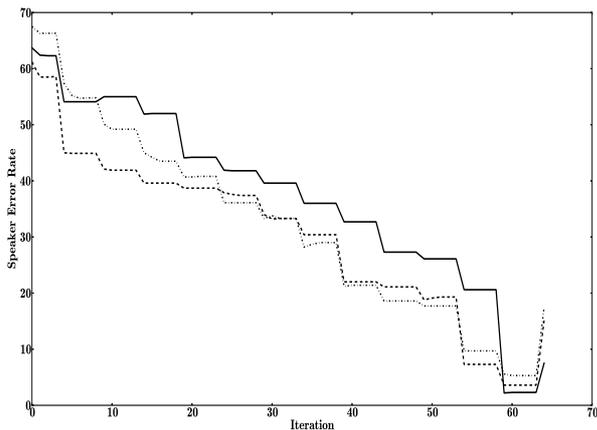
**Fig. 2.** The plot shows the reduction in Speaker Error Rate with each iteration of the KL-HMM system. Initially, there are 16 states and at each state, there are 5 iterations
