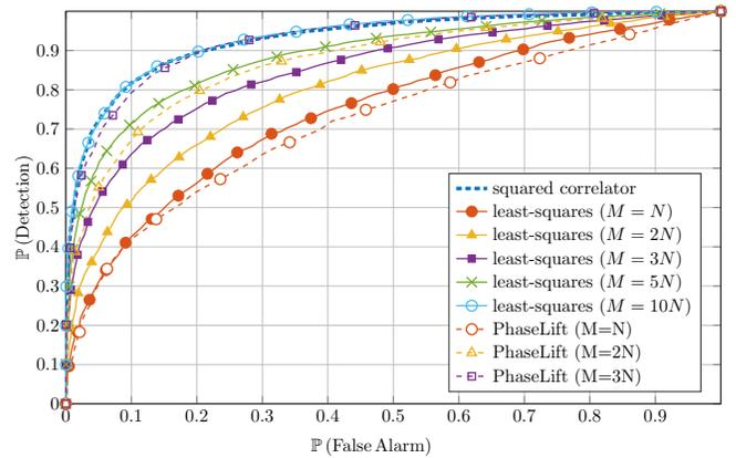
**Fig. 2:** Comparison of ROC curves for different values of  $M$  for our detector and for a reference method. Simulation parameters are  $N = 10, A = 2, \sigma^2 = 1$ . Simulations for our method are averaged over 10000 independent trials. PhaseLift simulations are averaged over 5000 independent trials.
