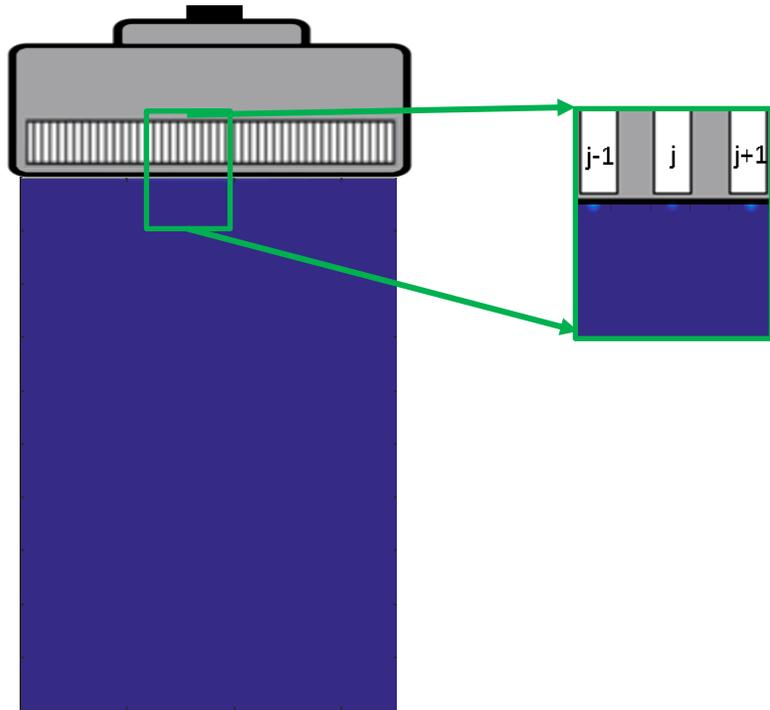
$$a_j(t) = \sum_{k=1}^{N_{pwi}} a^k(t) * \delta(t - t_j^k) \quad k - \text{plane wave index}$$
