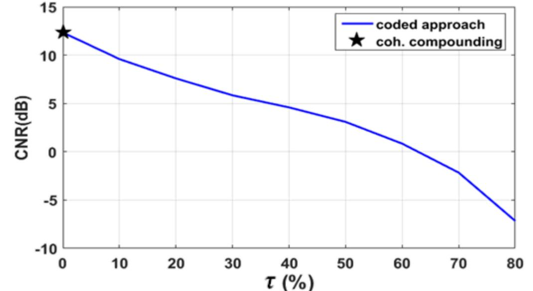
**Reducing the observation time adds a Perturbation Zone, that makes the system ill-posed thus the CNR drops**
