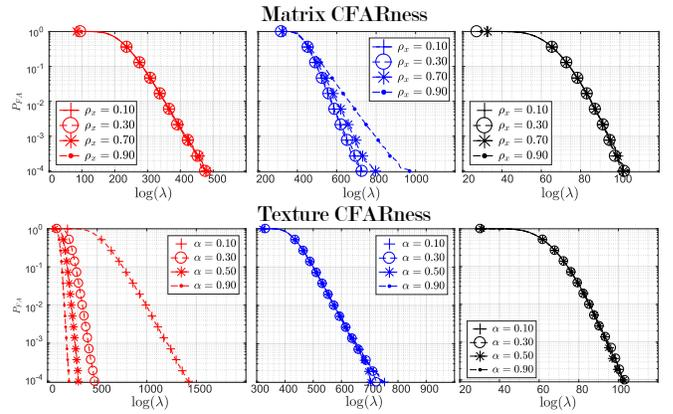
**Fig. 2.**  $P_{FA} - \lambda$ . Left =  $\hat{\Lambda}_G$ , Middle =  $\hat{\Lambda}_{lrt}$ , Right =  $\hat{\Lambda}_{glrt}$ .  $p = 10$ ,  $N = 25$ . Top:  $\alpha = 0.3$ ,  $\beta = 0.1$ . Bottom:  $\rho_x = 0.3$ ,  $\beta = 0.1$ .
