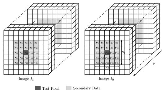
**Fig. 1.** Description of the problem. A sliding window of  $N = N_1 \times N_2$  observations  $\mathbf{x}_{i=1 \dots N}$  and  $\mathbf{y}_{i=1 \dots N}$  is used to compute the ratio for the test pixel.
