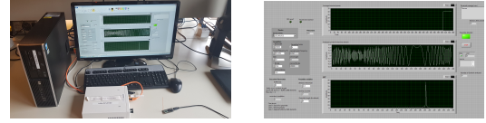
Fig. 4: Implementation set-up and the received LoRa signal.
