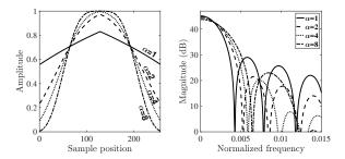
**Fig. 4**. Illustration of the shapes of proposed window with different values of  $\alpha$  and a window length of L=256.
