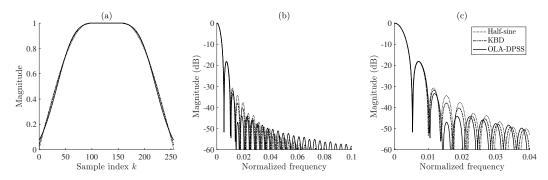
**Fig. 6.** Illustration of low-overlap versions of (a) the half-sine, KBD and proposed OLA-DPSS windows, (b) their spectral responses and (c) responses focused on the central region. Window length is L=256, overlap length is T=64, KBD has  $\alpha=4.25$  and OLA-DPSS has  $\alpha=5$ .
