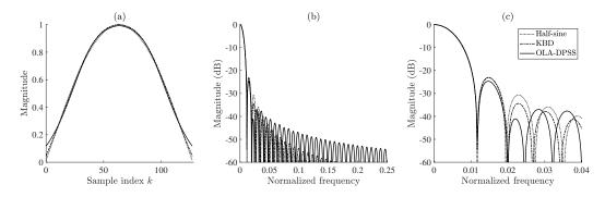
**Fig. 5**. Illustration of (a) the half-sine, KBD and proposed OLA-DPSS windows, (b) their spectral responses and (c) responses focused on the central region. Window length is L=128 and KBD has  $\alpha=4.25$  and OLA-DPSS has  $\alpha=2.75$ .
